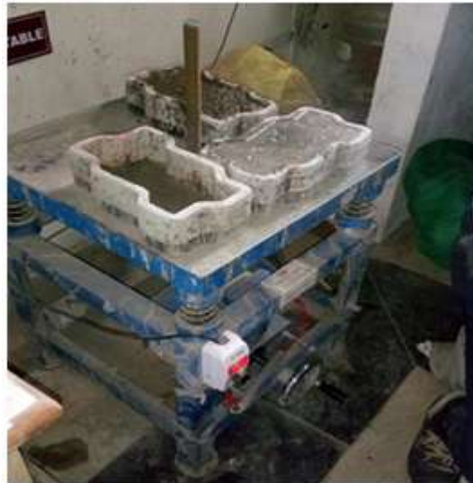
Fig.4. VIBRATING OF CONCRETE
